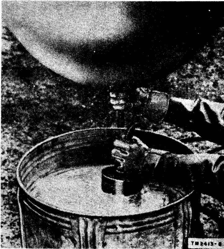
Figure 8. Hydrogen Generator ML-303/TM in operation.
